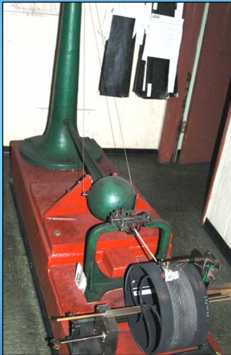
Ferndale's Bosch-Omori seismograph. The Washington, DC recording of the 1906 earthquake was made on an identical instrument.
