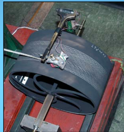
Ferndale's Bosch-Omori seismographs were built around the time of the 1906 earthquake and originally operated at Mare Island in San Pablo Bay. In 1933, the two horizontal instruments were installed in Ferndale. You can see them at the Ferndale Museum, Shaw & 3rd Street.
