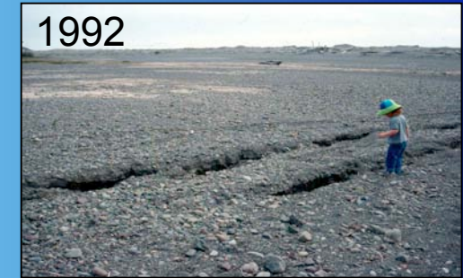
Liquefaction was observed along the Mattole River (above left) and locally in the Eel River Valley in 1992. In 1906 it was much more dramatic and widespread.
