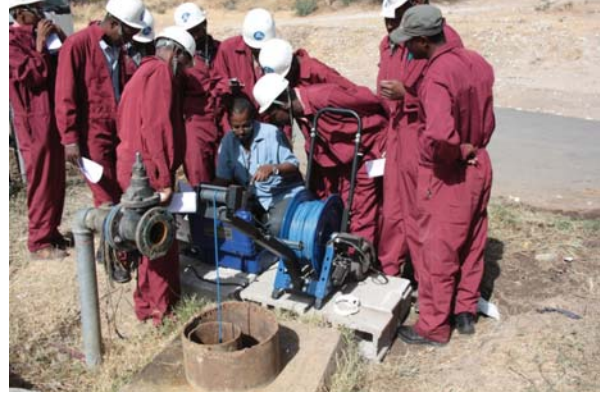
Trainees observing inside the well with a borehole camera (well diagnosis and well rehabilitation course).
