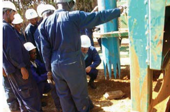
Demonstration for trouble shooting using the locally manufactured fishing tool by a Japanese expert.
