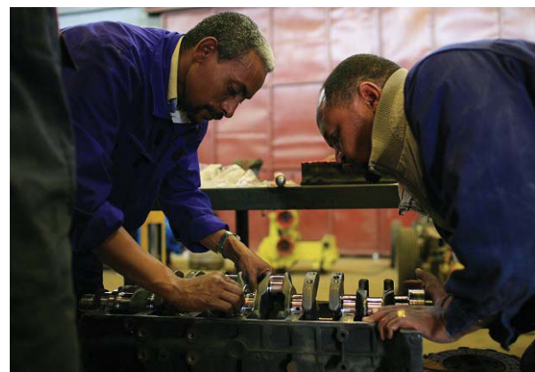
Practical training overhauling an engine for the mechanical engineering instructors.
