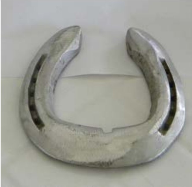
ILLEGAL Rolled toe
