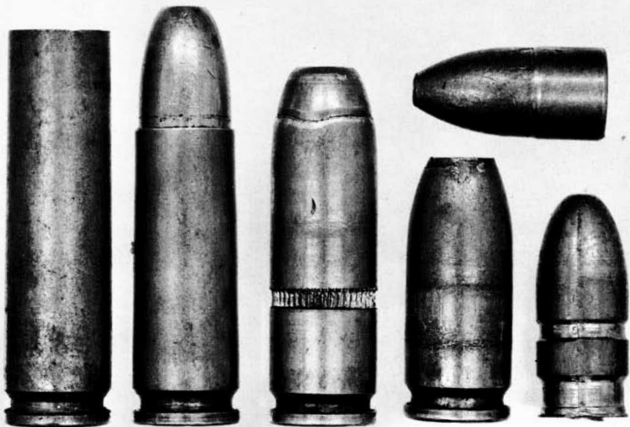
Left to right: .30 Carbine case; same but shortened and partially filled with lead core and topped with an issue .30 bullet to make a 275-grain .35 bullet; 230-grain S.P. swaged in Hemp die from .30 Carbine case with .30 half jacket over top a la Silvertip; 190-grain plain S.P. swaged from .30 Carbine case; lead and H-J bullets used for cores and tips.
