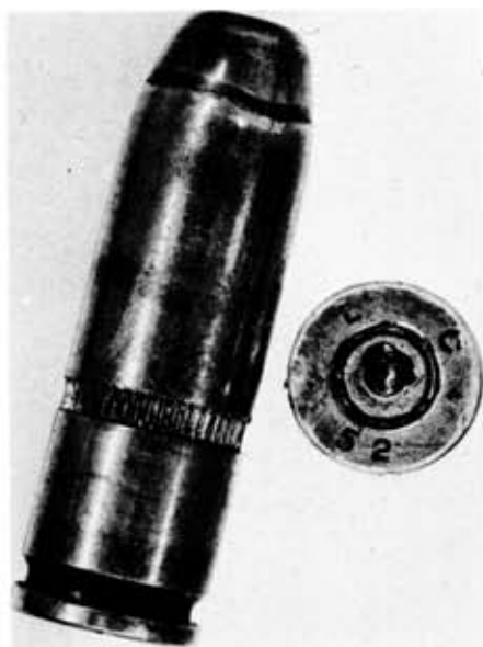
Above, a .35 caliber bullet swaged from .30 Carbine case. Half-jacket is placed over the lead nose to protect it. Cannellure is rolled in after swaging. Note case headstamp in the bullet base.
