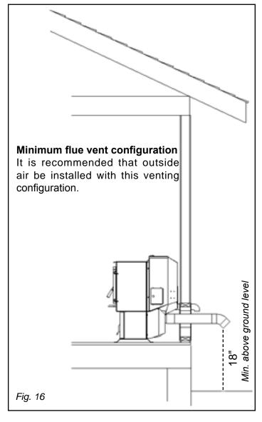
DO NOT INSTALL A FLUE DAMPER IN THE EXHAUST VENTING SYSTEM OF THIS UNIT.
