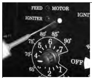
**Combustion Motor Speed Control**
