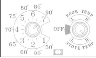
Fig. 20: This setting will produce continuous maximum heat output with the distribution blower at full speed.
