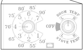
Fig. 22: Room Temperature Mode: This setting will produce a room temperature of 70 degrees with the distribution blower at medium speed.
