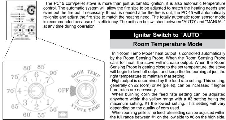
Fig. 19: Room Temperature Mode: This setting will produce a room temperature of 70 degrees with the distribution blower at medium speed.
