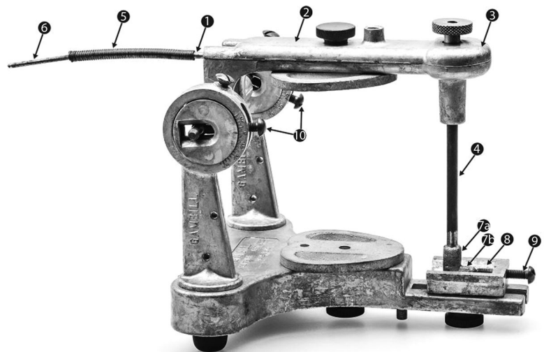
Figure 25 The Gambill Articulator, 1928. The grinding apparatus notwithstanding, this articulator may have been more competitive on the market if Gambill had chosen higher grade materials for its construction; however, there is no evidence to suggest that he made any improvements in that regard. A ridged shaft (1) is located within the upper member (2) extending forward to (3) where it is connected to the worm-gear and pinion system that rotates the incisal pin (4). Posteriorly, the ridged shaft is attached to a long flexible shaft (spring) (5) from which extends a large diameter copper wire (6). The power source was most likely a belt driven, variable speed handpiece. The tip of the incisal pin had vertical (7a) and horizontal (7b) units that engaged the horizontal V-shaped incisal guide (8). Incisal screw (9) and condylar screws (10) established centric position.
