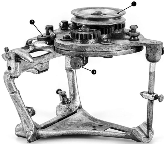
Figure 3 House "Occlusal Grinding Device for Articulators." Unlike the model illustrated in the patent letter, this model can be mounted on the Snow "New Century" and "Acme" and the Kerr articulators using the additional holes (2) for the retaining screws.
