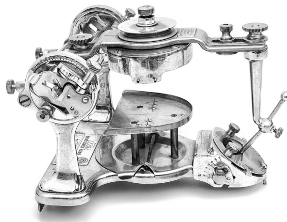
Figure 8 The House Articulator (1927). The occlusal grinder’s mechanical components were sealed in a metal casing for protection and lubrication.
