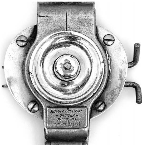
Figure 9 A top view detail of the House occlusal grinder showing the pulley and metal casing. Even though House received patents on his grinding devices, he did not patent any of his articulators. 3
