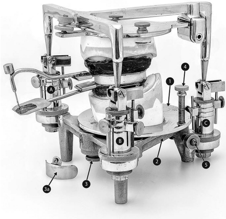
Figure 15 Side view of the Stansbery "Tripod." The maxillary and mandibular casts are mounted with Stansbery's extraoral tracer. Note that there are two anterior controls (A & B), through which the extraoral tracer extends, and one control (C) centered posteriorly. The upper member is in the shape of a "T," while the lower controls form a triangle.
