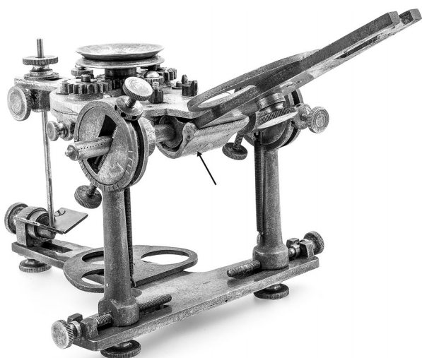
Figure 6 The Wadsworth articulator (1925) with the grinder in place. This is a posterior lateral view of the special attachment (arrow) used to secure the grinder to the horizontal condylar post.
