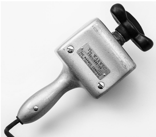
Figure 32 The Warwec “Equilibrator,” W. Ross Stromberg, 1960. This device was introduced to the profession as a means to generate vibration of the mandible to refine complete denture occlusion in the mouth.
