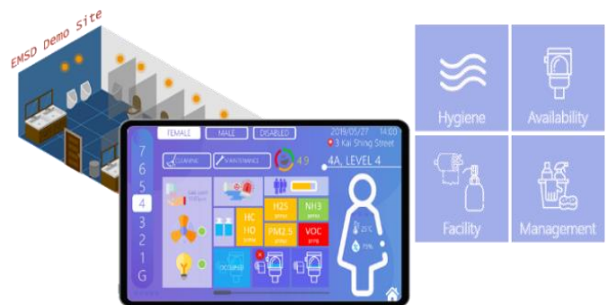
Fig. 4 - Smart toilet management system
