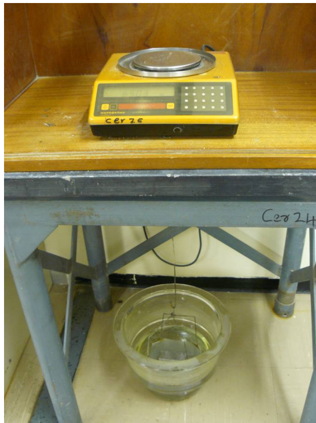
Figure 2: Laboratory Archimedes setup
