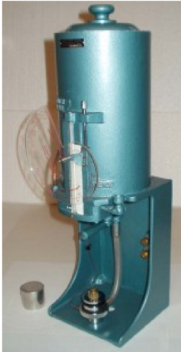
Figure 10: Ridsdale permeability apparatus
