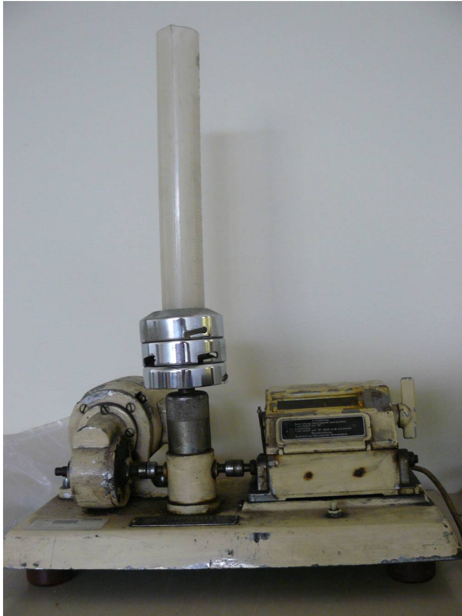
Figure 8: Grain or powder Tap Density apparatus
