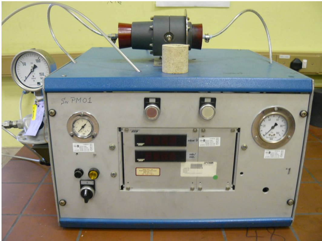
Figure 11: Refractories permeability tester
