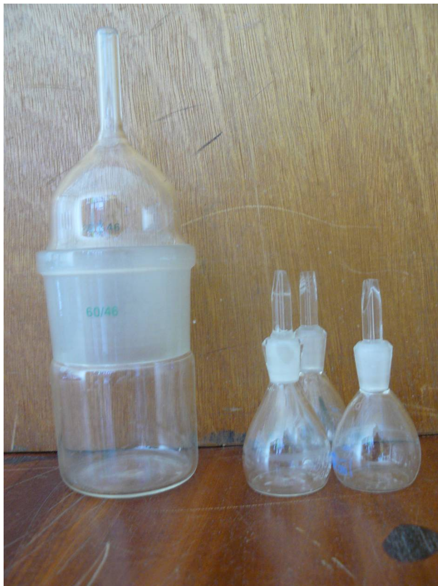
Figure 4: Bulk Pycnometer (left) and SG Bottles (right)
