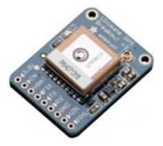
The breakout is built around the third generation MTK3339-based module which has external antenna support and Pulse-Per-Second
