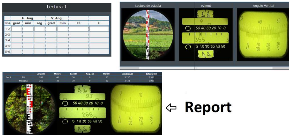
Figure 3. This traverse module is based on a Pentax Fx-1 theodolite. The readings are shown in the righthand side of the image while the report is shown in the lower left part of the image
