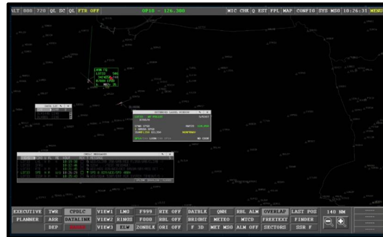
1st data link application - CPDLC - Controller-Pilot Data Link Communication
