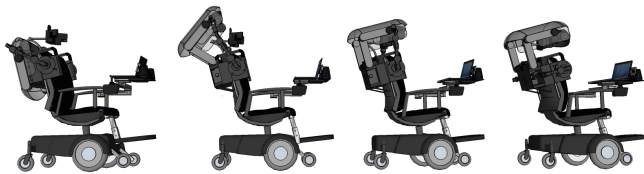
Fig. 7. 3-D rendering of the iChair raising its roof. Left to right: Robotic Arm Assistant (RAA) reaches back and unlocks the Retractable Roof (RR); 2 Mount-n-Movers rotate assisted by 2 12V servos and aided by the robotic arms; RR locks into position and the heads up display (HD) rotates into the user's field of view.
