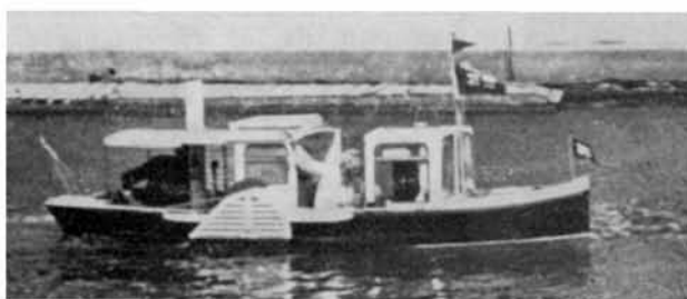
Firecrest, the 15' steam-driven paddleboat built by David Garrick. She is powered by a single coal-fired boiler developing one quarter horsepower.
