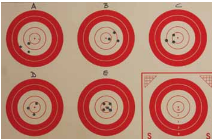
A demonstration target of sighting-in with three-shot groups. A is the original setting, B shows too much adjustment, C is too far left and D is about right. E is what we are looking for!
