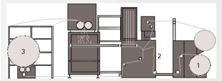
Example: Stitch-bonding machine with chopper (glass chopping device)
