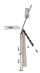
6 - The needles descend to knock-over position and the previous loop slips from the needle stem over the needle hook. The loops in the needle hooks are interlaced with the previous loop, thus producing a new course of loops.
