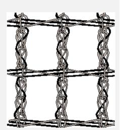
The structure shown in the illustration is used as shading net and can be produced in various shade grades.
