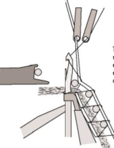
The knitting elements of this Raschel machine with web feed facility are engineered to place the two vertically entering reinforcements (warp/weft) onto the nonwoven.
