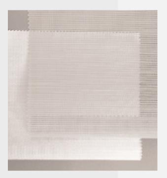
Heat-reflecting and shade-providing warp-knitted sun-protection fabric. The special properties of this structure are: economical production, high strength and high dimensional stability. No sagging of the fabric and good rolling behaviour due to stretched weft yarn layers. The porous structure prevents heat accumulation and ensures additional shading. The aluminium coating serves for sun reflection and heat insulation.
