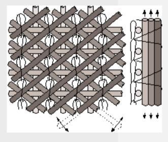
A multi-axial multi-ply fabric demonstrating the two diagonal yarn sets in addition to the bi-axial yarn sets created by the mislapping guide bar (warp or ST-yarn) and the magazine weft insertion system (weft).
