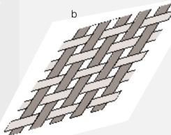
Unlike woven fabrics, multi-axial multi-ply structures have a high shearing strength under diagonal forces
