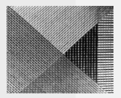
Four yarn layers placed in perfect order each on top of the other. Each layer shows the uniformity of the noncrimped parallel yarns interlaced by stitches. The structure is dimensionally stable in all directions:  $+450/-450/0^{\circ}/90^{\circ}$ .
