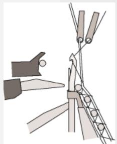
Knitting area of Raschel machine with magazine weft insertion
