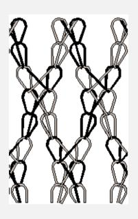
Another way to produce an open structure is to form loops continuously on the same needle and to interlace them laterally at certain intervals.
