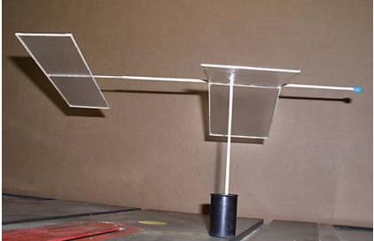
Balance the glider at the position shown on the plans by adding clay to the front of the glider (fuselage nose).
