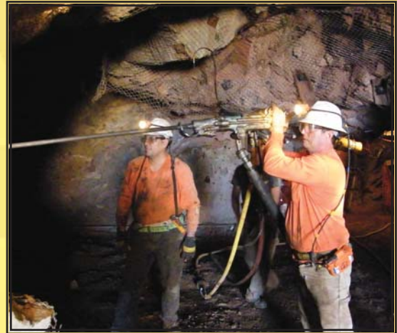
Drilling blast holes on the face inside the mine. (L to R) Ruven Avina & Alfie Pereyda.
