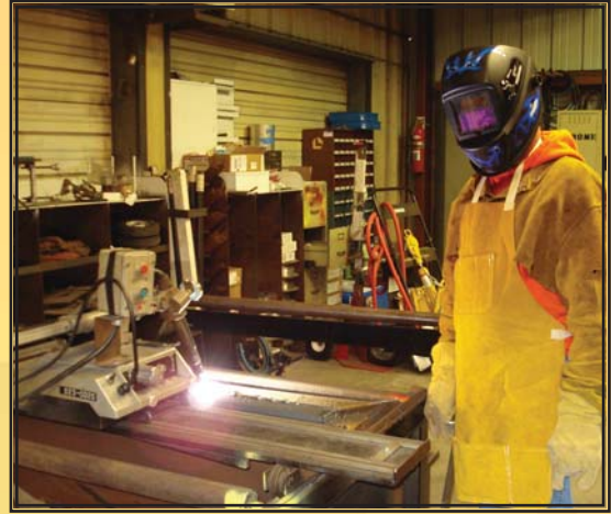
Cutting test panels with the plasma cutter machine.
