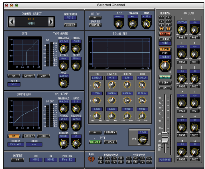
Settings for CHs 12-19 Compressor Settings
