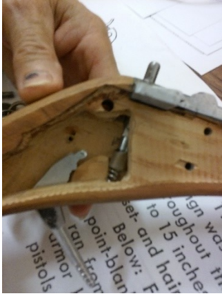
Release mechanism and barrel installed in stock.
