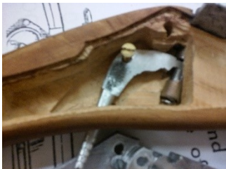
Trigger installed in release mechanism
