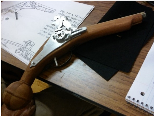
Lock plate installed in finished pistol
