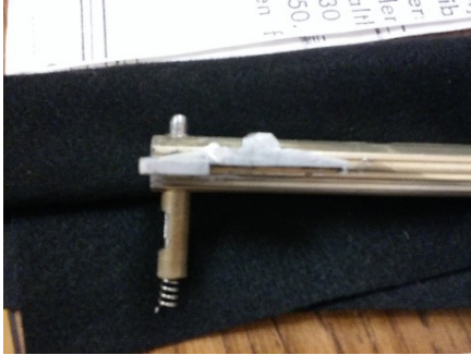
Release mechanism installed in barrel with pan and pan cover
