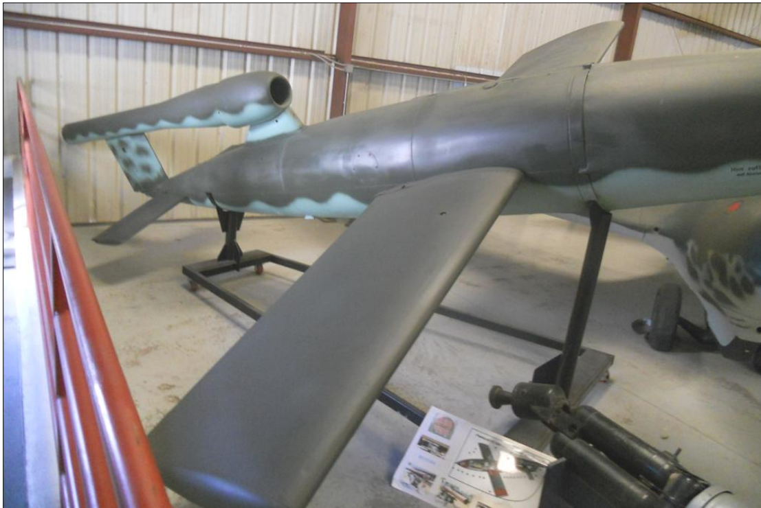
Flying bomb with pulse engine (Planes of Fame Museum Chino CA; photo rs)
