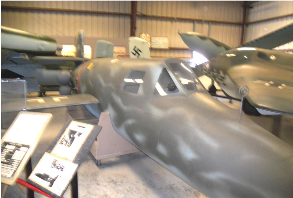
Bachem Natter, manned rocket for vertical start, 1944 (Planes of Fame Museum, Chino)
