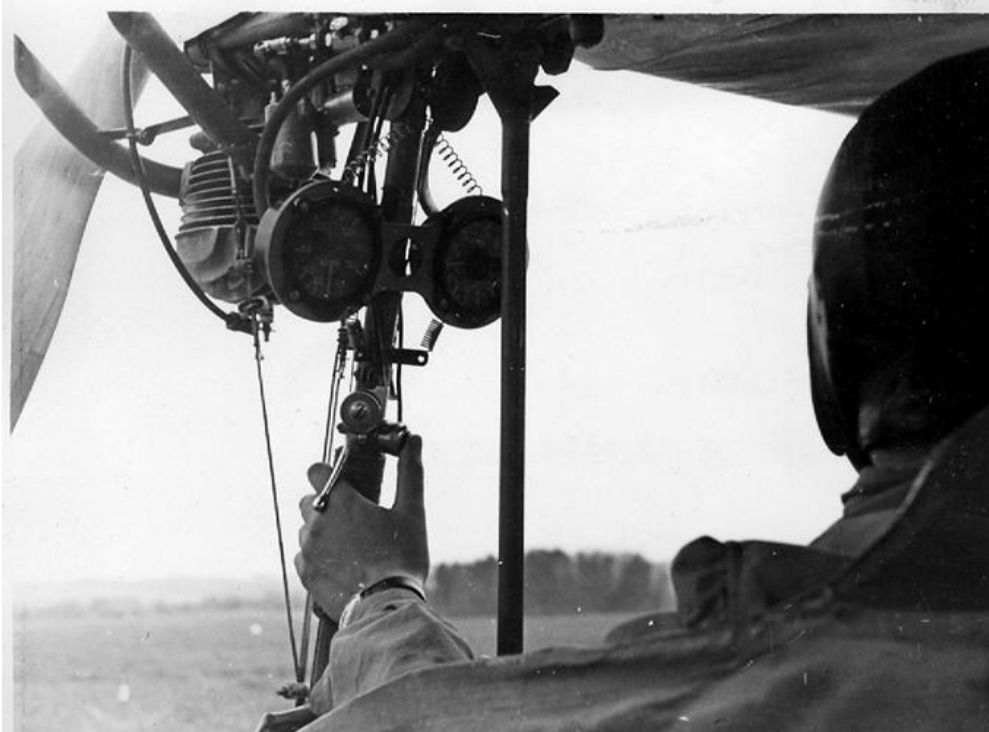
Glider with Zündapp motor; speed + altitude meters; hanging stick
