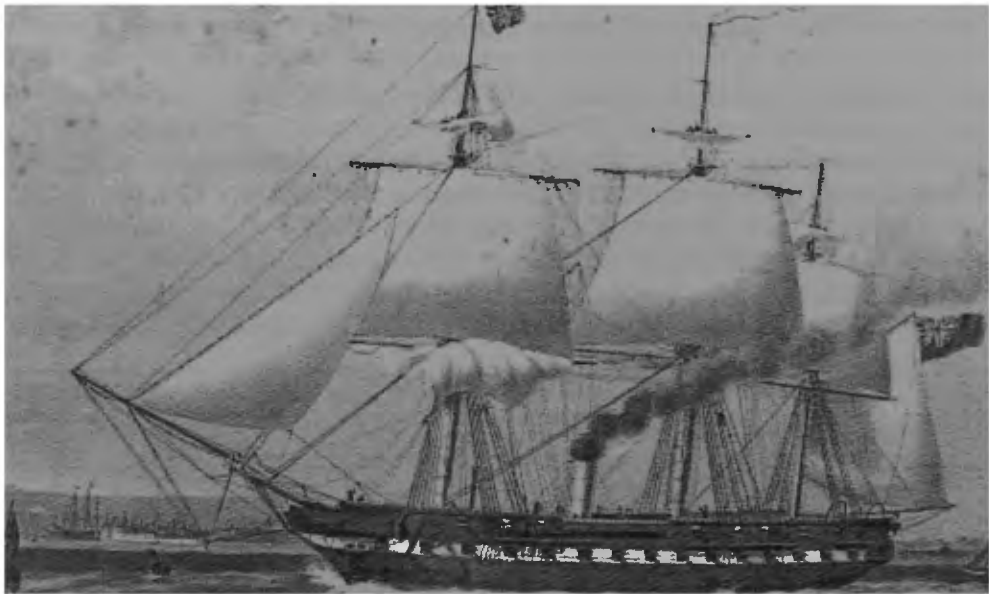
A lithographic portrait of the steam frigate Arrogant , one of the first screw-propelled major warships, to which Robert FitzRoy was appointed in 1849.
