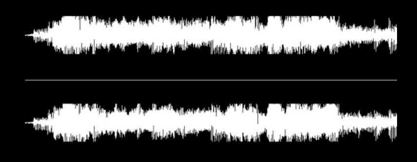
to the same song, remastered in 2006, we find the dynamic range has gone from 13 to 7. The new version has some crunch distortion during the chorus due to clipping of the bass, especially on the word "fall,"
