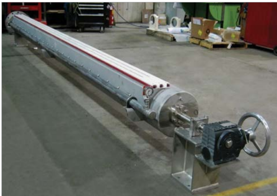
Figure 3: Typical Uhle Box of a Paper Machine (Vacuum Connection on Back Side)
