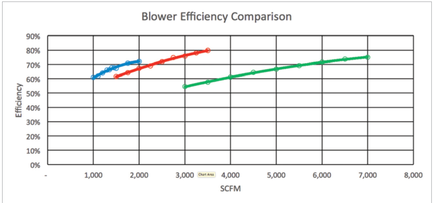
Figure 4: Example Blower Efficiencies
