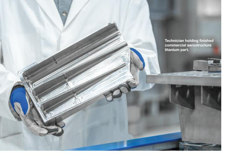
RPD's buy-to-fly ratio (the weight ratio between the raw material used for a component and the weight of the component itself) is much lower than traditional forged and machined components. "Customers will need to buy less titanium and machine less titanium away. It's just plain math," Fuller says.
