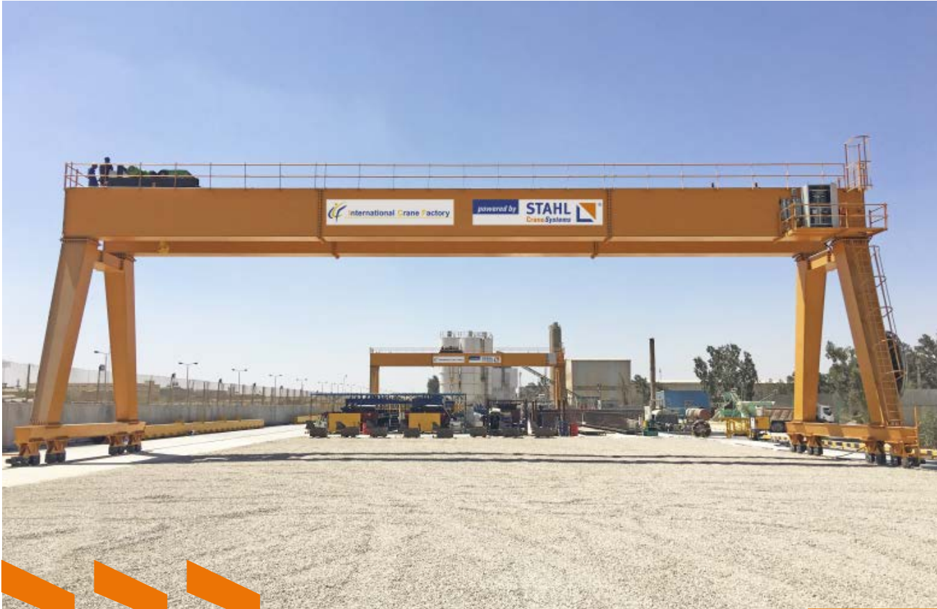
The two AS 7 twin hoists lift concrete parts weighing up to 140 tonnes.
