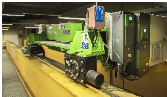
The frequency inverter enables careful lifting and lowering of the loads.
