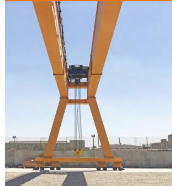
As the ropes of the twin hoist run in opposite directions simultaneously, the load is lifted and lowered without any sideways movement of the hook and can be positioned exactly.
