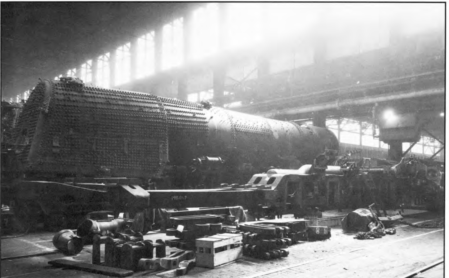
Frame of S1b #6007 in foreground, boiler and frame of #6008 to rear. Erecting Shop, American Locomotive Company, Schenectady, N.Y., 1945. Alco Historic Photos.
