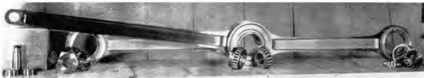
Fig. 8—Light-weight locomotive main and side rods of Timken design and made from Timken High Dynamic Steel
