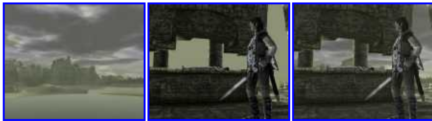
1. Distant view rendering ("SuperLow", described later) 2. Foreground (only the high and medium models) 3. Combination of (1) and (2) using the Z-buffer mask.
