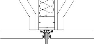
For all NEW/LIGHT ceilings we strongly recommend the use of our double-layer system. The upper layer's main function is to be a dust barrier and insure the longevity of the aesthetic of the visible layer. The upper layer can be a clear membrane or a translucent membrane as well.
