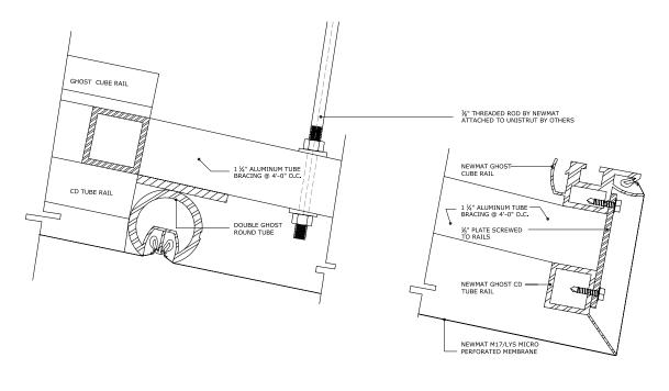
This structure was built in our metal shop, separated into six segments that were shipped to the jobsite, elevated into place and reassembled. The membranes were then stretched over it.
