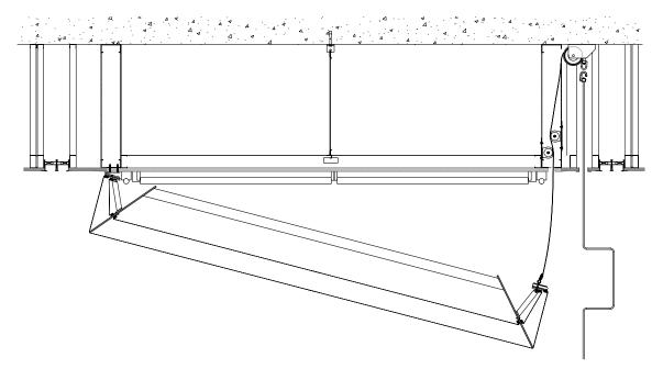
While this project specified a mechanical pulley system to open the NEW/LIGHT box to access the lighting, on other similar projects we have provided electrical winch systems to achieve the same access by simply pressing a wall switch.
