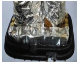
Figure 4 Spring fastening method on outside of test samples
