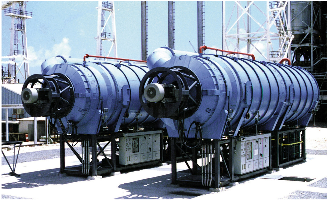
Figure 3: 2 x MVC 1,250 operating since 1990 in an Alumina Smelter
