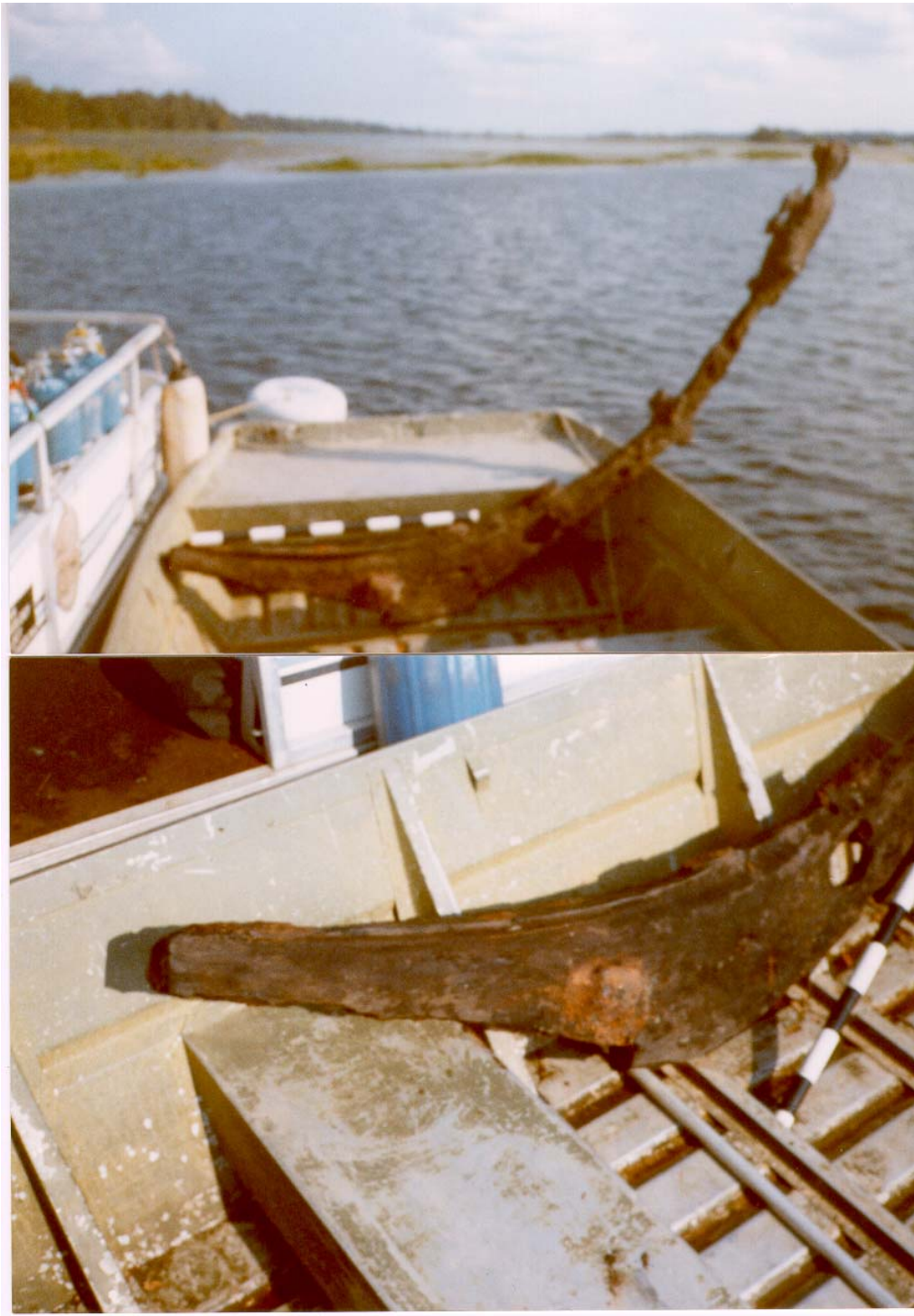
Figure 9. Two Views of the Stem (photographs taken October 2000 by Sue Vezeau). The complete stem is shown at top and a detail of the base and the keel scarf is shown in the lower photo.
