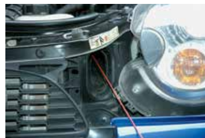
Don't use Seafoam in the air intake, it will seep through the plastic tube, not making it to the engine.
