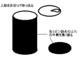
2. Insulator: Cut off top of the PET bottle at the level of 3 cm taller than the can.
