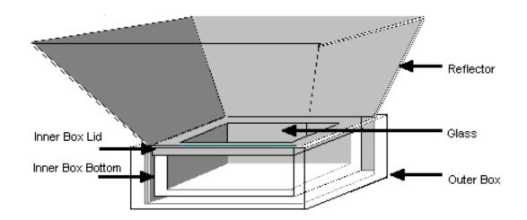
Figure 6: Diagram of complete solar oven.
