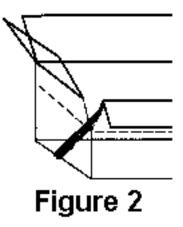
Glue aluminum foil to the inside of both boxes and also to the inside of the remaining top flaps of the outer box. Don't waste your time being neat on the outer box, since it will never be seen, nor will it experience any wear. The inner box will be visible even after assembly, so if it matters to you, you might want to take more time here. Glue the top flaps closed on the outer box.
