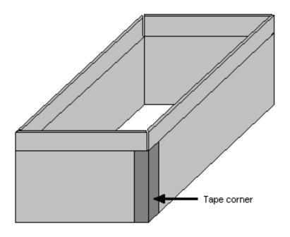
Figure 13. Fold the 5" wide strip of cardboard into a rectangle. Tape the ends together.
