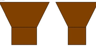
the reflector illustrated Figure 6 when fastened together. The inner box is rectangular, so two of the reflectors that surround it are wider than the other two. The illustration in Figure 7 shows one of the wider reflectors, with a width of 20" at the narrow base, on the left. The reflector on the right is one of the two narrower reflectors, with a width of 14" at the narrow base. The instructions will cover cutting each size separately.
