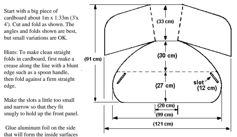
To set up, lay panel flat with shiny side up. Fold up front and back parts and fit back corners into the slots in front.
