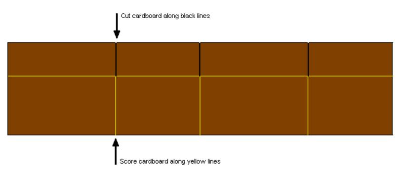
Figure 11. Cut and score the 5" strip of cardboard for the inner box lid.
