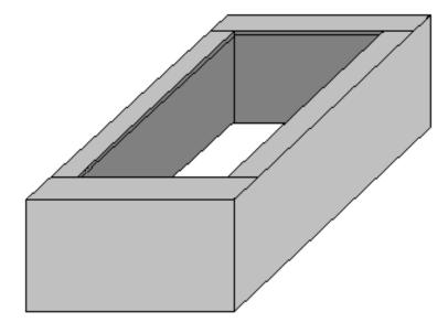
4. Fold the top flaps down, and tape into place. Figure 14 shows the completed inner box lid with its open center, which will allow the sunlight into the oven.
