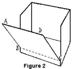
To make an ROB, start with a rectangular, rather tall, cardboard box (see below for dimensions). On one of the broader sides, draw a horizontal line (BC) about two inches above the bottom (figure 2) and cut the seams along AB (stop at B) and DC (stop at C). Fold down the front panel ABCD using BC as a hinge. Stack a few rectangular pieces of cardboard in the bottom of the box, to raise the floor level up to the level of BC. The Reflective Open Box Solar Cooker
