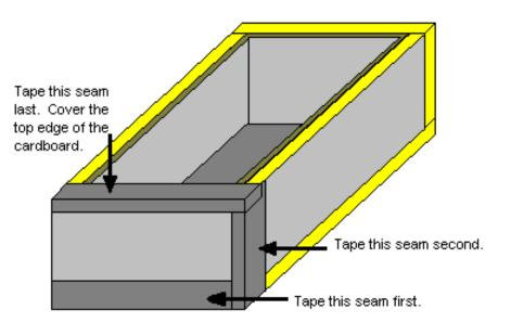
Figure 9. Tape the sheathing in place with aluminum foil tape.
