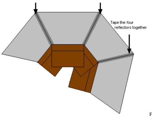
Figure 17. Tape the four reflector pieces
