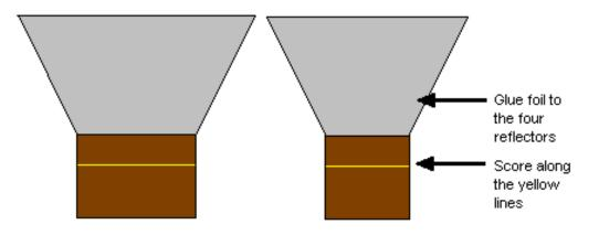
Figure 16. Glue foil to the four reflectors. Score the cardboard along the yellow line, 5" below the base of the trapezoid.
