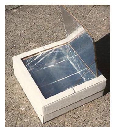
2. Fold an extra cardboard piece so that it forms a liner around the inside of the base (see Figure 2).
