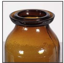
Figure 9 – Four-piece mold (North American Glass)
