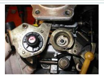
Re-fit the black electrical thingy on top of the springs (A/C idle up actuator?). Note there is a slot in the bottom, which needs to line up with the throttle shaft. Moving the base plate may assist in getting it located
