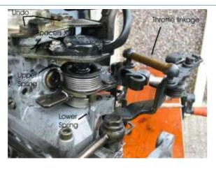
Unhook the top spring. Get the tipex/felt pen to hand. Press down on the base plate to keep it still while undoing the nut. Keep holding it down and lift off the top spring exposing the base plate. Mark the base plate so you can install it on the same spline. If lined up wrong it will either not idle or idle way to fast but can be adjusted when on the car. Unhook the lower spring and lift off.
