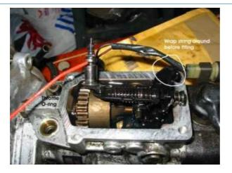
Replace the top cover seal. And the o-ring on the throttle shaft.
