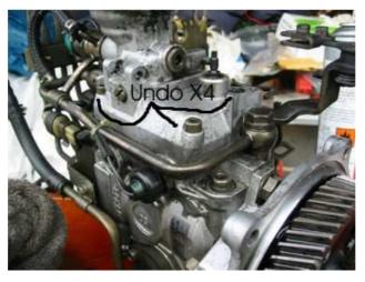
Undo the 4 allen key bolts (5mm allen key) holding the top on. They are all the same length.
