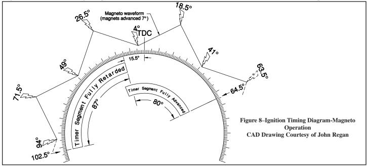
reflect the timing relationship attained by advancing the magnets on the flywheel by 7 degrees as indicated on flywheel drawing T-701-C. The spark symbols show the points where the ignition coil will fire on the magneto current output with respect to piston travel. Each of these locations is logically separated by 22.5 degrees.
