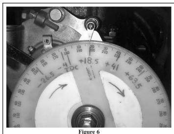
Figure 6-Degree Wheel Mounted on Crankshaft with Pointer
