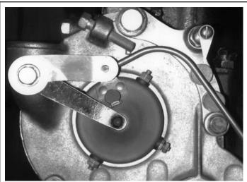
Figure 3-Timer Mounted on Engine Using Original Ford Adjustment Gauge Photo Courtesy of Steve Coniff
