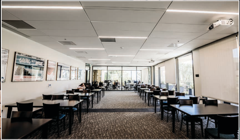
The renovated library has plenty of glass and natural light, which affected projection choices. Projectors that produce 6,500 lumens, like the one seen here, are laser-light-source devices. They replaced the bulb-light-source projectors used previously throughout Pepperdine classrooms.
