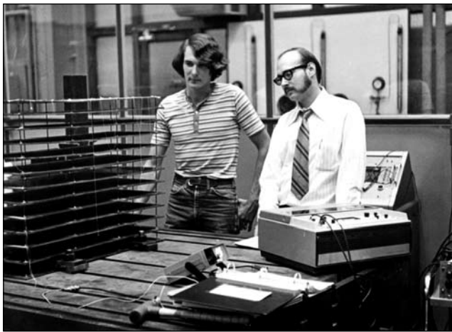
Figure 13. Step input test of building model, student project group: Jerry Nessler (left) and Ray Zimmerman (1972).
