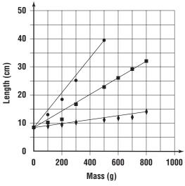
Width of rubber band: • 2 mm • 4 mm • 7 mm
