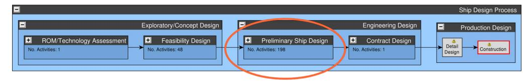
The process shown in this document depicts the Preliminary Design stage of a surface combatant. The Exploratory and Concept Design stages are generally subsets of the activities included in Preliminary Design. The set of Preliminary Design activities represents the foundation for expanded activities in Contract Design, and Detail Design and Construction.
