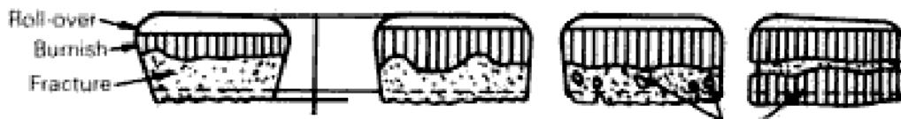
Drawing 5.2.1: Correlation between die-cut edges of Product and Clearance.
