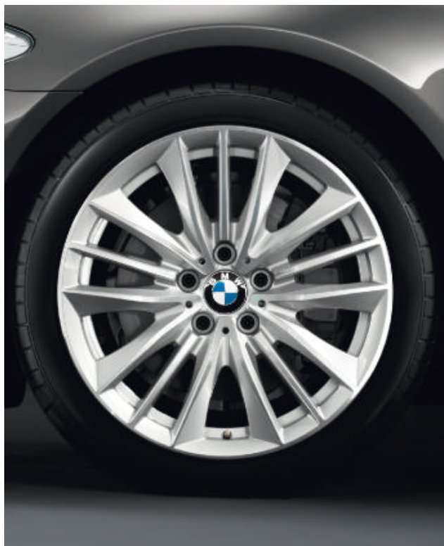
□ BMW light-alloy wheels W-spoke 332 with mixed runflat tyres, 8.5 J x 19 inch, 245/40 R 19 tyres at the front, 9 J x 19 inch, 275/35 R 19 tyres at the rear.
