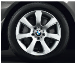
□ BMW light-alloy wheels star-spoke 330 with mixed runflat tyres, 8 J x 18 inch, 245/45 R 18 tyres at the front, 9 J x 18 inch, 275/40 R 18 tyres at the rear.
