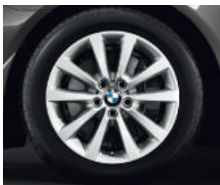
□ BMW light-alloy wheels V-spoke 328 with runflat tyres, 8 J x 18 inch, 245/45 R 18 tyres (standard on 550i).
