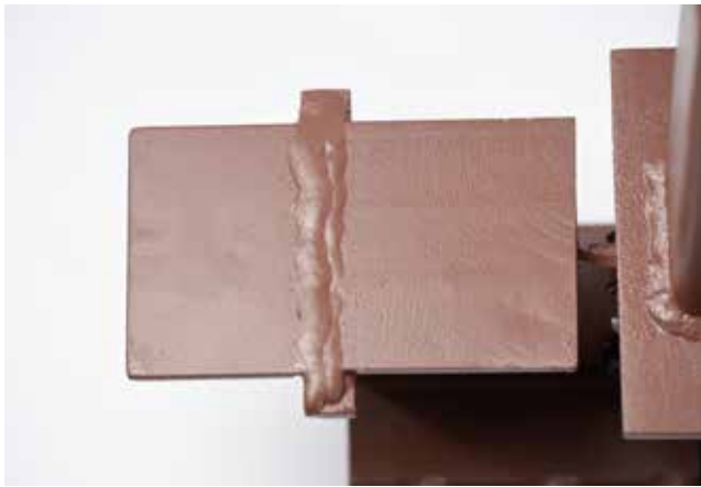
▲ SSS: Weld backing bar in place and non-uniform welds.
