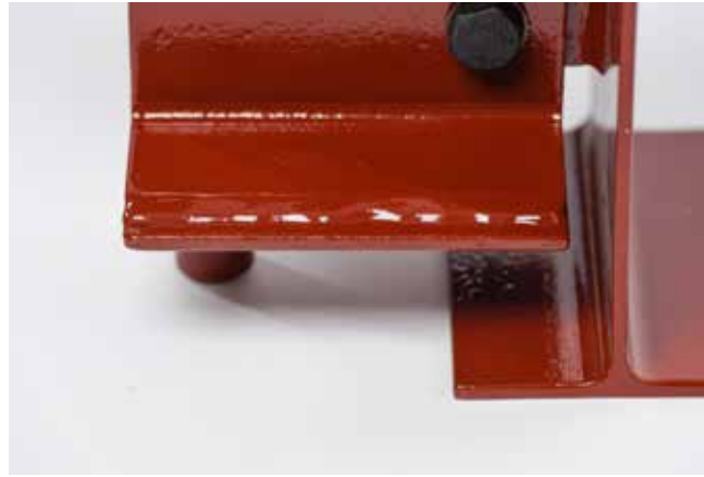
▲ AESS 1: Continuous weld appearance.
