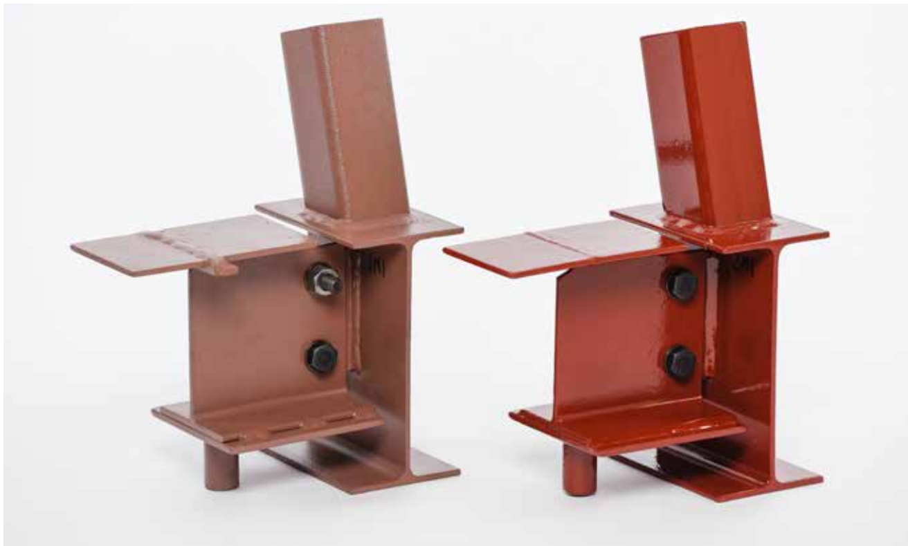
▲ Left: Standard structural steel (SSPC-SP2). Right: AESS 1 (SSPC-SP6).
