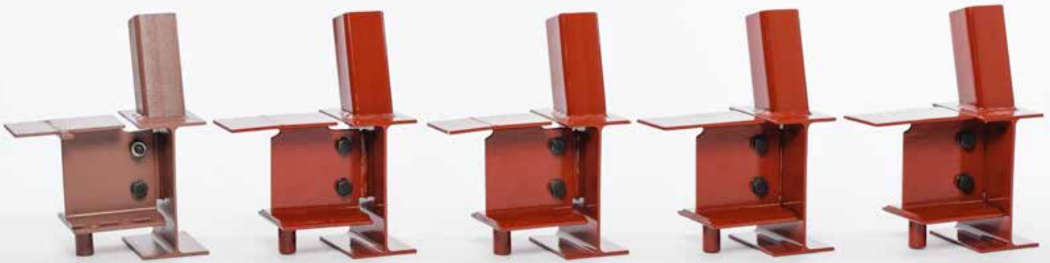
▲ From left to right: Standard structural steel (SSS), AESS 1, AESS 2, AESS 3 and AESS 4.
