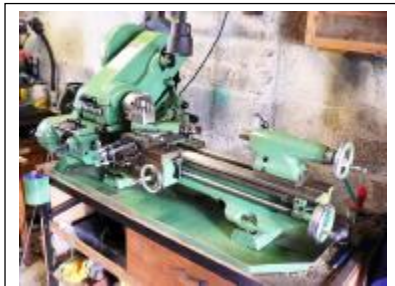
A typical model engineers lathe, the Myford 7. Note the lack of provision for using any coolant.
