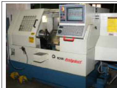
Photo courtesy of Hardinge Inc. A modern CNC lathe with the safety guard open.
