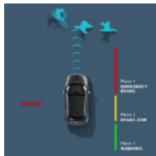
Autonomous Emergency Braking: with pedestrian and cyclist detection
