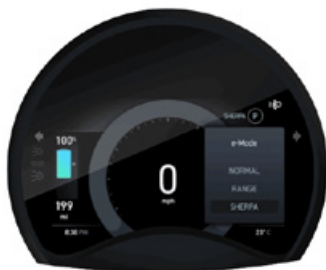
Sherpa Mode: the energy saving mode that saves your car's energy by limiting speed and acceleration
