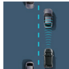
Adaptive Cruise Control: sets and keeps a safe distance vehicles in front
