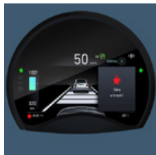
Attention Assist: detects driver fatigue and advises you to take a break
