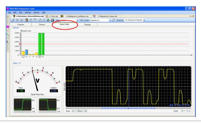
Signal Quality Window: Oscilloscope
