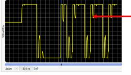
You can see the reflections in the oscilloscope display of master 2 while connected at test point Slave 71.
