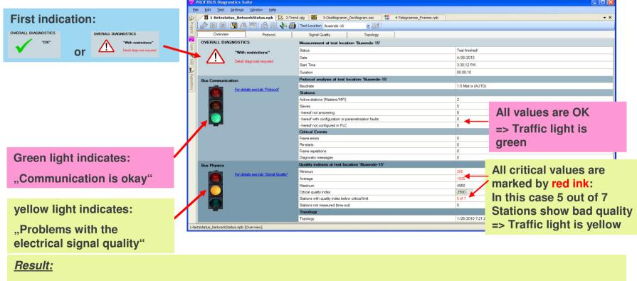
Measurement from this end indicates bad signal quality. Click on "Signal Quality" (link or tab) for more details
