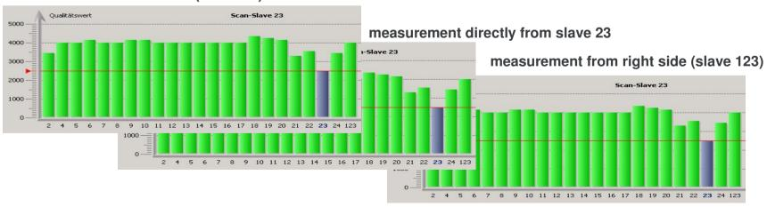
Case 5: Bus-termination is not powered correctly
