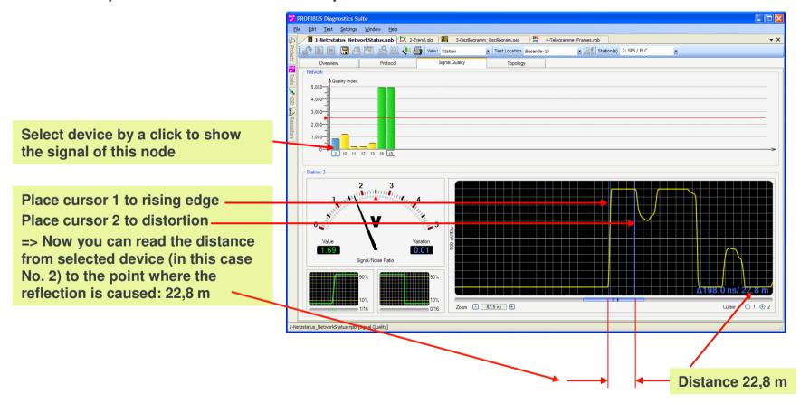
Signal Quality Window: Oscilloscope
