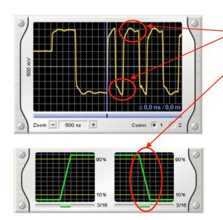
signal blurred only some drops in signal due to reflections bad signal edges
