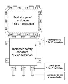
If the cable glands and the cables used are certified as unique and indivisible part of the equipment (enclosure), it is not required the conformity, according to what is written in paragraph 10.6.2 of the standard 60079-14 (see Note 2 of paragraph 10.6.2 of the same rule).
