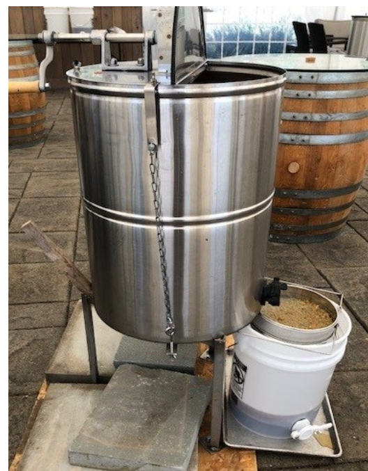
Extractor with strainer & 5-gallon bucket below
