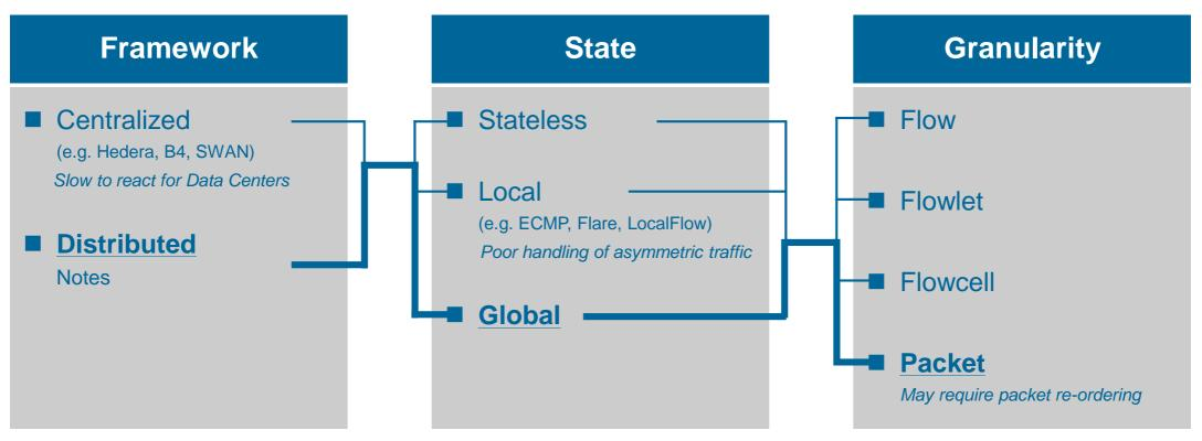
LPS = Packet Spraying + Endpoint Reordering + Load-Aware
