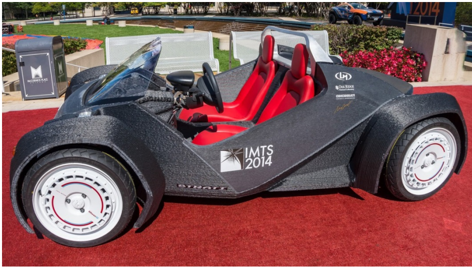
Figure 5.4. Local Motors 3D printed car body
